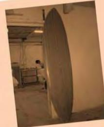
Cured boards are then lightly sanded and prepped for finishing
