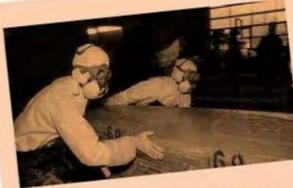
The mould is closed over the board, fully wrapped in cloth, sandwich-material and resin. The board will now cure at 50° for 1 hour under 3 tons pressure
